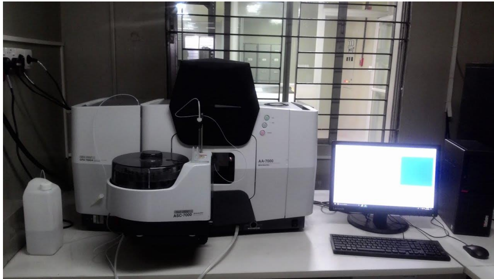
Figure (1). Diagram of Atomic Absorption Spectrometer used in the present study.
