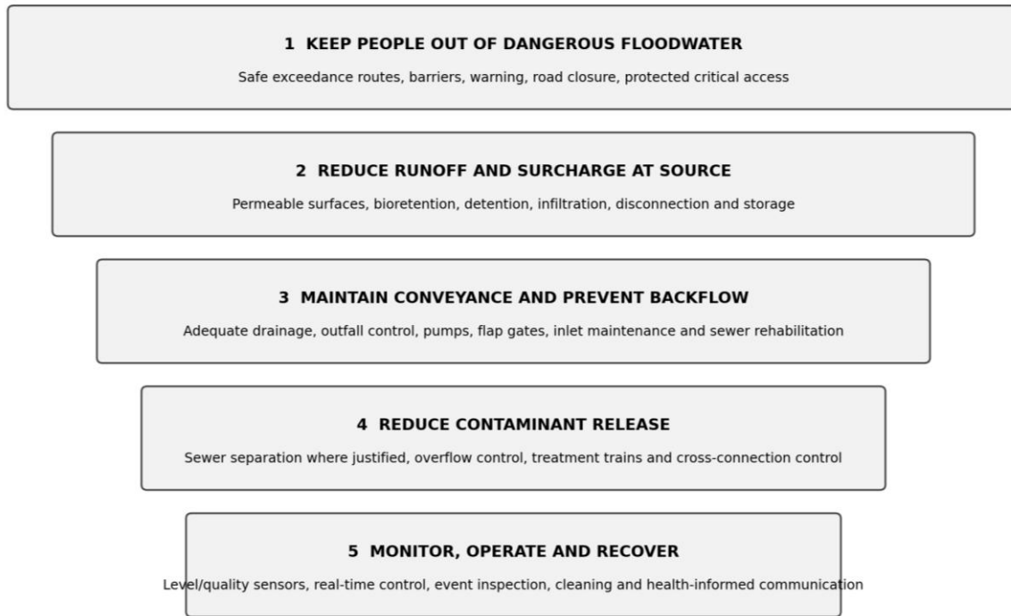
Figure 3. Proposed hierarchy for health-protective urban drainage and flood-contamination management. Original synthesis by the authors.
