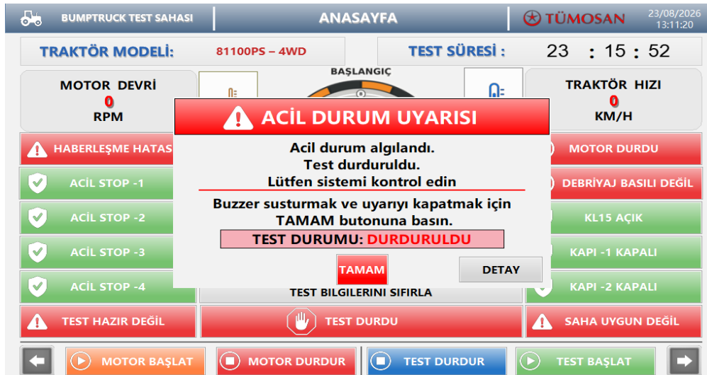
Figure 6 - HMI Emergency Screen
