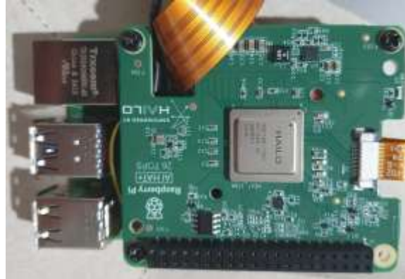
Figure 3.4. The Hailo 8 that used as an AI accelerator
