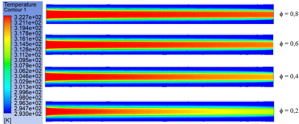
Figure 9. Temperature contours for different porosity values at Re = 250 and T_{in} = 50^\circ C ( L/D = 0.071 ).
