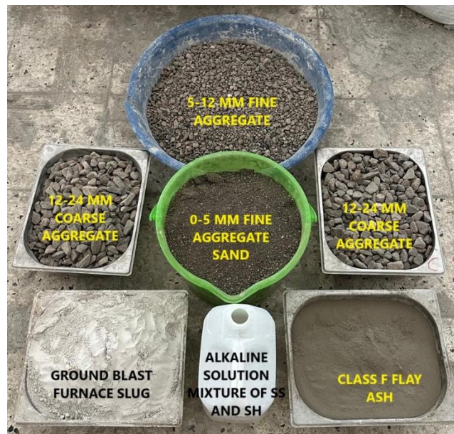
Figure 5: Geopolymer Concrete Components
