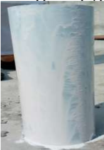
figure 2.5 PVC pipe white petrol paint coating
